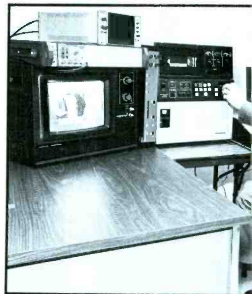
The author, with some of WNEV-TV's newly purchased equipment. Shown (left to right) are a video waveform monitor, a Panasonic AU-300 \frac{1}{2} -inch VCR, a Convergence ECS 103B editing console, a Panasonic AU-300, a Convergence SE-100 editing effects/switching system, an Ikegami HL-83 camera and a bolt-on Ikegami HM-100 M Format portable field recorder.
