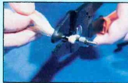
Fiber-optic connector being attached to a fiber cable using Kevlar as a strain relief beneath the crimp sleeve.
