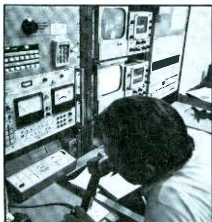
The ENG command center operator remotely controls antennas at the pickup sites.
