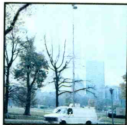
The LOOK live vehicle with its 46-foot mast extended.
